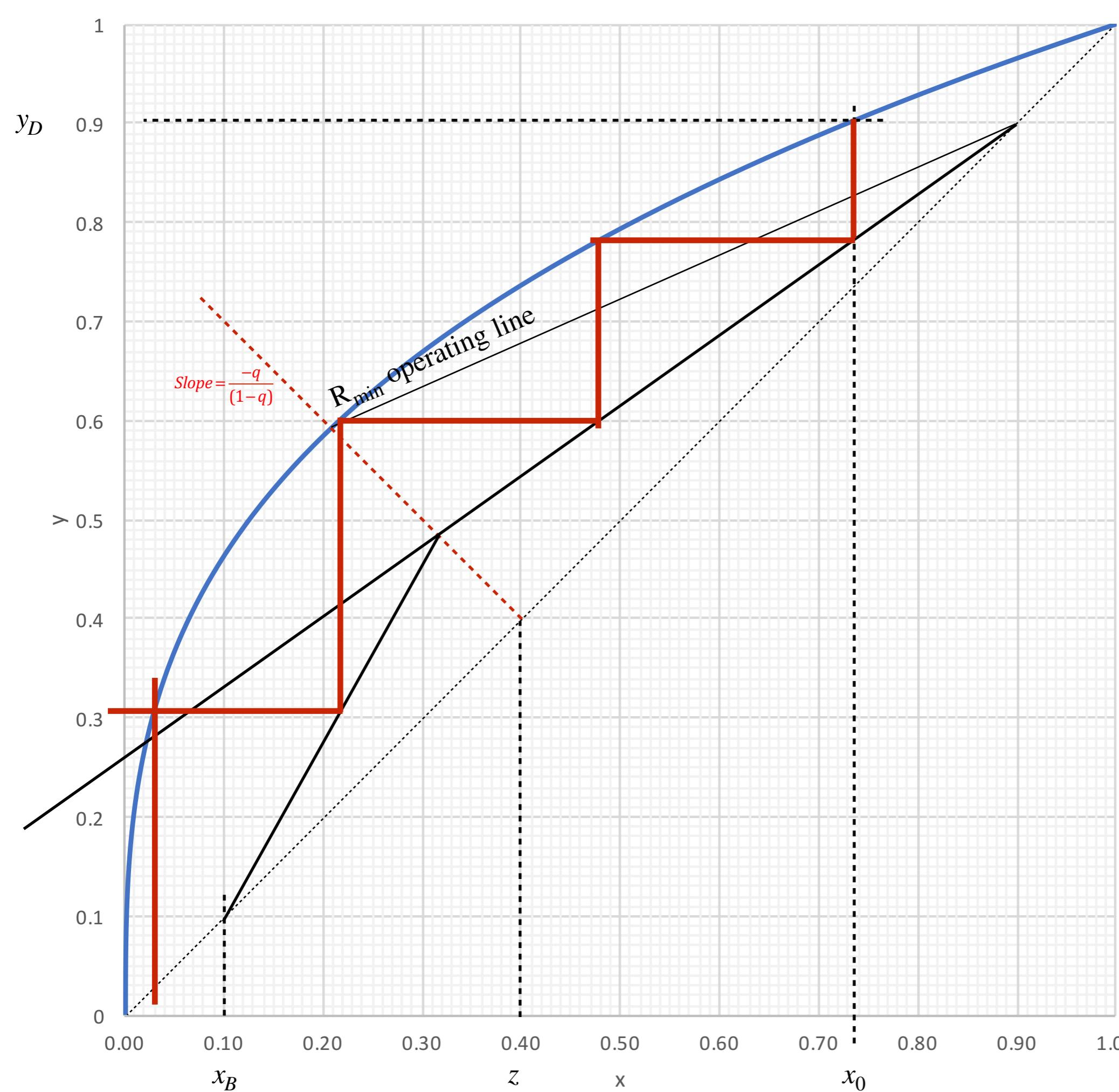
$$\frac{R_{min}}{R_{min} + 1} = \frac{0.90 - 0.59}{0.90 - 0.21} = 0.45$$
